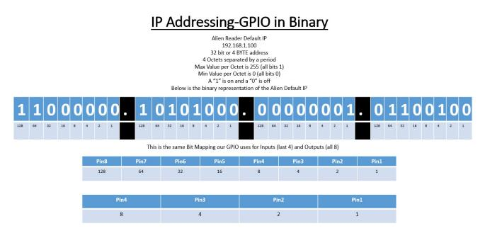
Numbers 1 through 128 represent the value of that bit placeholder when it is set to "ON"
