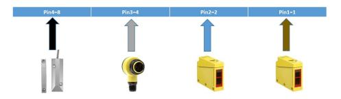
2 Banner Q60's connected to pins 1 and 2, 1 Banner T18 connected to pin 3, 1 magnetic sensor connected to pin 4 Simply add up the pin/s for the desired start or stop triggers
